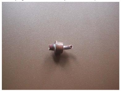
Using the air nozzle, we ascertained that an angle approximately degrees was necessary on the outlet pipe and the hole approximately half way between the end of the whistle and voice slot itself, with the outlet hole just off the inside body of whistle the tube. Andrew's test piece was 1/8" made with copper pipe approximate 0.080" i.d. and proved unsuccessful.
