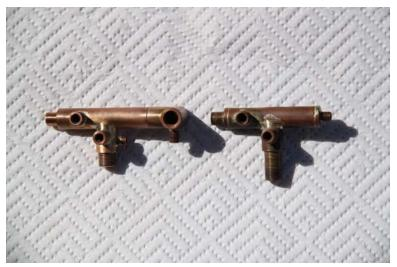
Back in September, and after much deliberation debate. and а new manifold was made as neither Andrew nor I were quite happy with the original one. The slightly redesigned manifold allowed for the pressure gauge take off be moved to the vertical upright and an improved blower valve to take its place,
