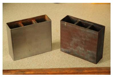
The two aforementioned base pieces were soldered with varying amounts of success and these have since been milled flat. The final job to do was to remove the thousands of machine marks with dubious amounts of emery paper, which has left a brilliant smooth finish.
