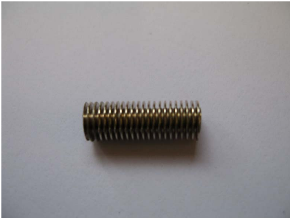
(Picture 1 – The bellows used for operating the gauge gear mechanism)
