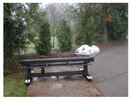
The main transporter has now been completed (**See Picture Left**), with the new bearing and gearbox fitted and duly sealed. The track section was then placed back in the vertical slides and it is now ready for action. One or two minor tweaks may need to be made as it settles in, but is a vast improvement on the knackered transporter that we had at the end of last season. The secondary transporter is now receiving attention, with 4x 8" stainless wheels turned
